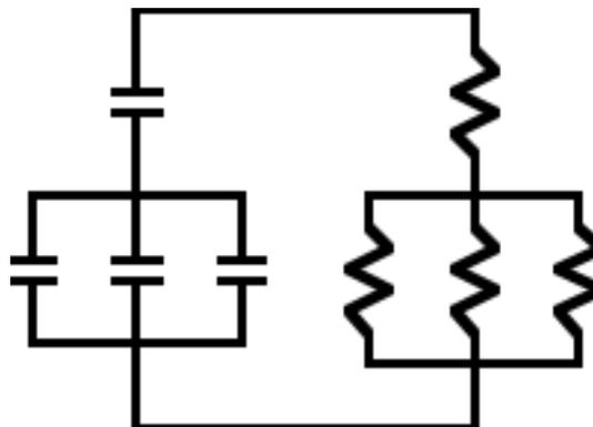
a) Find the equivalent capacitance and resistance and redraw the circuit using them. All C's are 3 milliFarad and all resistors are 1000 Ohms.
