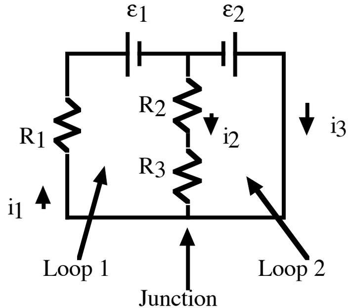
$R_1 = 100 \text{ Ohms}$ ,  $R_2 = R_3 = 75 \text{ Ohms}$ ,  $\epsilon_1 = 9 \text{ V}$  and  $\epsilon_2 = 6 \text{ V}$ .
