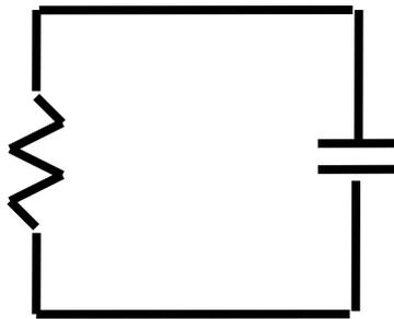
The capacitor is initially charged to a voltage of 12 Volts. It discharges through the resistor and reaches a voltage of 8 volts in 5s.
