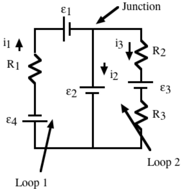
$R_1 = 200$  Ohms,  $R_2 = 300$  Ohms,  $R_3 = 400$  Ohms,  $\epsilon_1 = 40$  V,  $\epsilon_2 = 20$  V,  $\epsilon_3 = 10$  V,  $\epsilon_4 = 30$  V.
