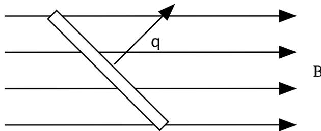
$$\begin{aligned}\Phi_B &= BA \cos \theta \\ &= B N a b \cos \theta \\ \theta &= \omega t = 2 \pi f t \\ \Phi_B &= B A \cos 2 \pi f t\end{aligned}$$
