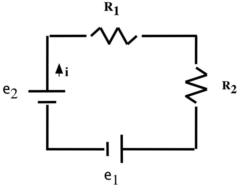
We can solve for the current by first assuming a current direction. We assume a current  $i$  as shown above. We begin our analysis path in the lower left hand corner and use the sign convention. Kirchoff's voltage loop rule yields
