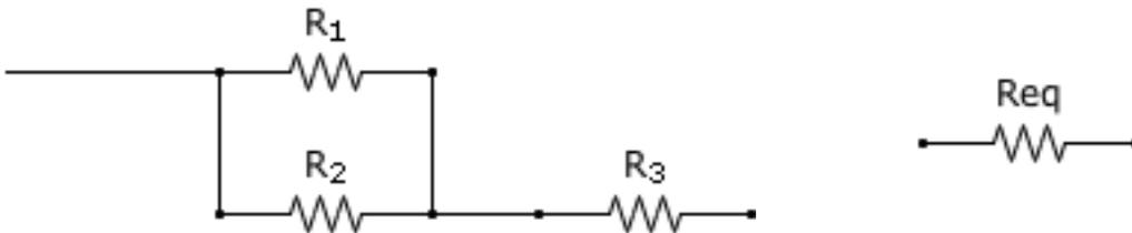
Here we combine  $R_1$  and  $R_2$  in parallel (to yield  $R = 2\Omega$ ). This equivalent resistance is in series with  $R_3$  and the final equivalent resistance is  $R_{eq} = 4.5\Omega$
