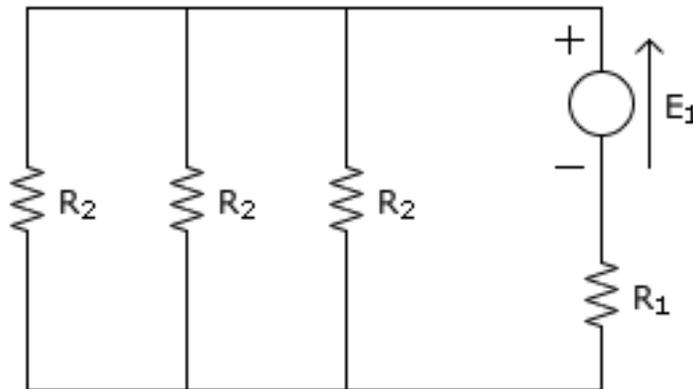
And find an equivalent resistance for the parallel R's.
