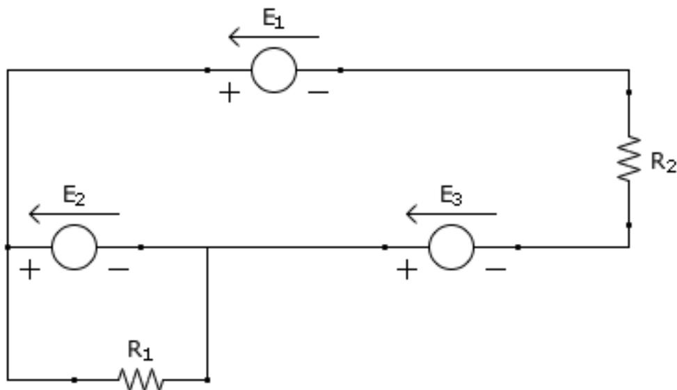
a) The current in resistor 1 is entirely determined by the potential difference across it--given by emf 2
