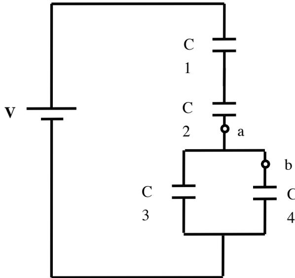
Since  $12\mu C$  passed through a , we know that the charge on both  $C_1$  and  $C_2$  must be  $12\mu C$  . We can compute the voltage across  $C_2$ .
