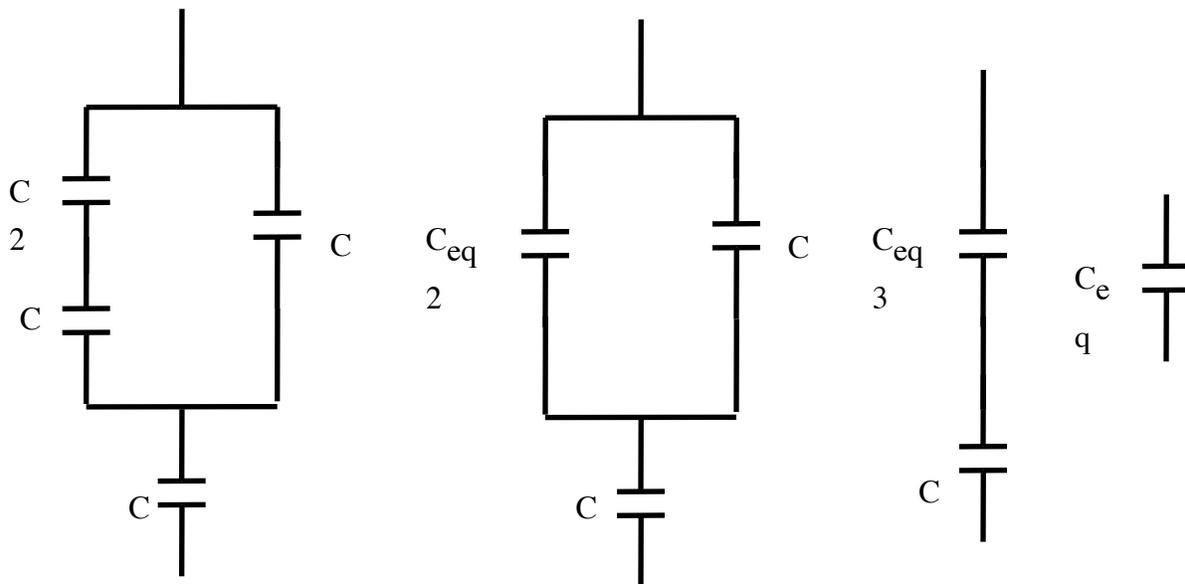
$$\frac{1}{C_{eq2}} = \frac{1}{C} + \frac{1}{C} = \frac{2}{C} \Rightarrow C_{eq2} = \frac{C}{2} = 5\mu F$$
