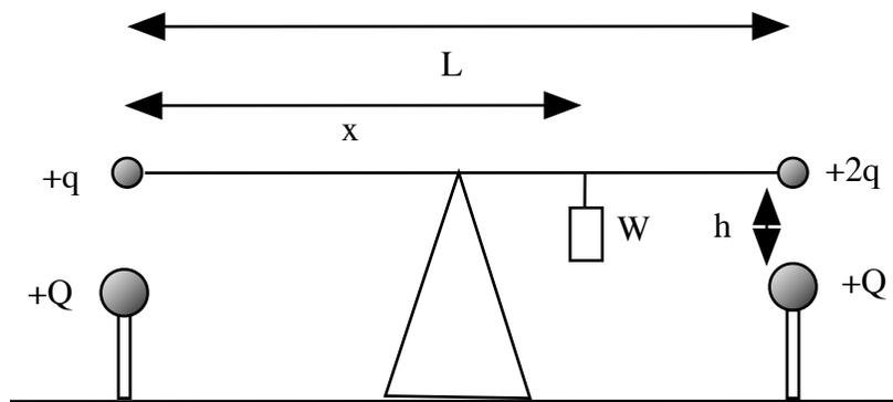
a) To proceed, we compute the torque about the central pivot. We will assume that torques that would cause clockwise acceleration are positive. Since the system is to remain at rest, the net torque must be zero.
