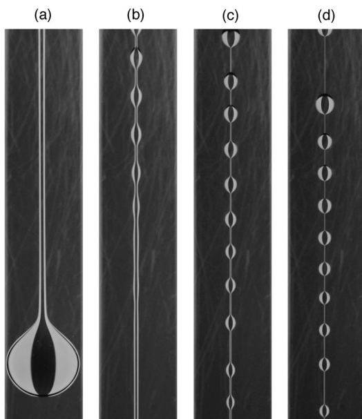
FIG. 2. Progression of the beads-on-string structure on a thinning filament of 12 mM CPCl/NaSal in PDMS oil. Each image size is 8.2 \times 1.3 \text{ cm}^2 ; times shown are (a) 3 min, (b) 4 min, (c) 5 min, and (d) 6 min.
