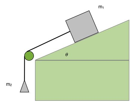
a) Draw the forces on each block and draw a free body diagram for each block.
