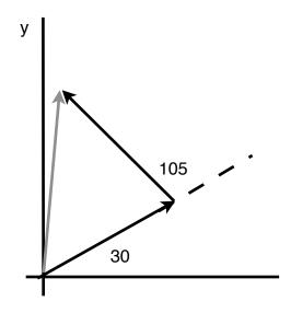
We need to write out the two vectors in component notation. To do this, we need to remember that we need to write each angle with respect to the positive x axis
