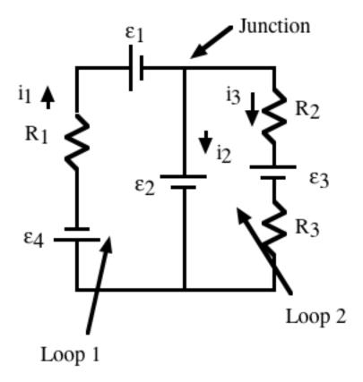
$R_1 = 200 \; \mathrm{Ohms}, \; R_2 = 300 \; \mathrm{Ohms}, \; R_3 = 400 \; \mathrm{Ohms}, \; e_1 = 40 \; \mathrm{V}, \; e_2 = 20 \; \mathrm{V}, \; \; e_3 = 10 \; \mathrm{V}, \; e_4 = 30 \; \mathrm{V}.$
