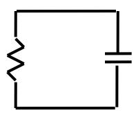
The capacitor is initially charged to a voltage of 12 Volts. It discharges through the resistor and reaches a voltage of 8 volts in 5s.
