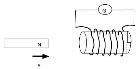
The magnetic flux rises to the right. The coil will respond to oppose this change in flux, so it will develop a current to produce a field to the left. A current will flow up the front face, causing the needle to deflect left.
