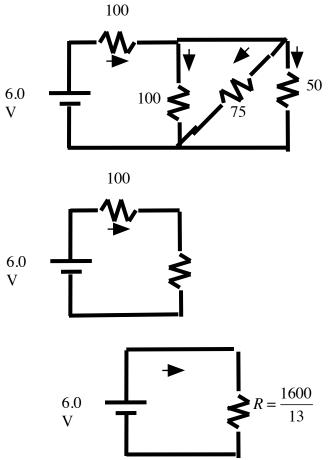
Now that we know the equivalent resistance, we can find the current that flows through the equivalent resistance. This is also the current through resistor 1.
