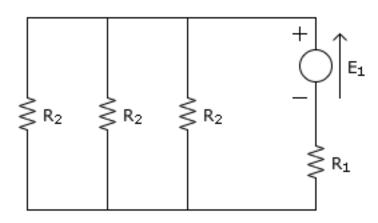
And find an equivalent resistance for the parallel R's.
