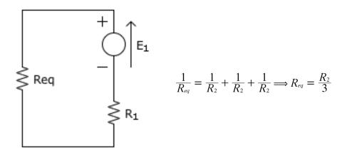
We can now find the current in the circuit. We can compute the voltage drop across the equivalent resistor now that we know V.
