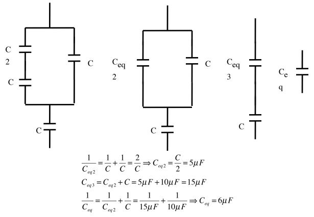
Now that we know the progression of substitutions, we can start with the final equivalent capacitor and work backward to find the charge on  $C_2$ . We know that the voltage across the equivalent capacitor is 10V.
